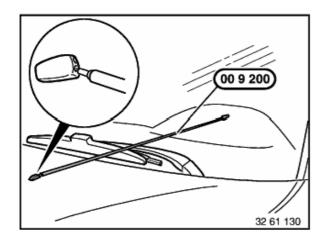
If necessary, adjust left or right spray nozzle with special tool  $00\ 9\ 200$  .
