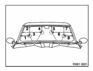
Mark contact points with adhesive tape on windscreen. Actuate windscreen washer system.
